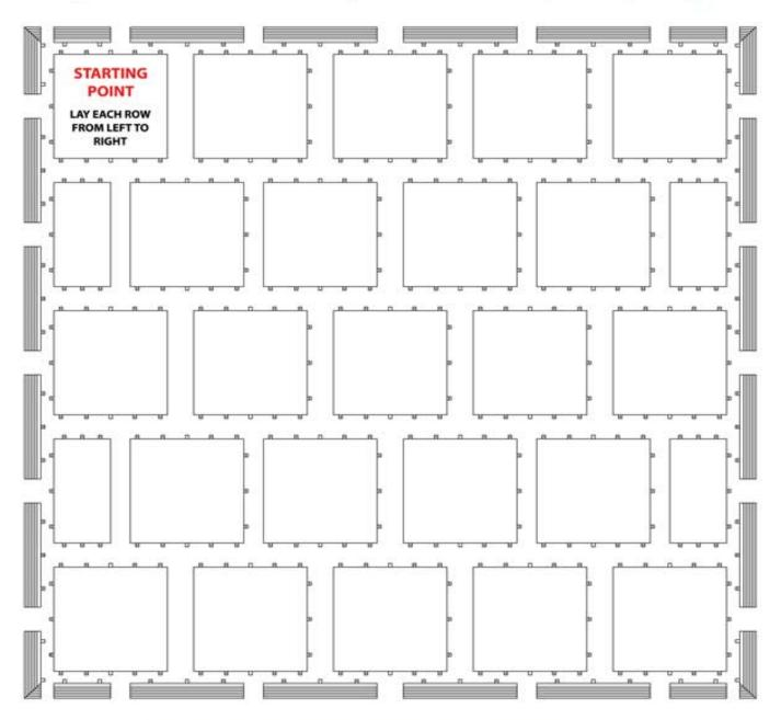
COMPONENTS: 23 FULL PANELS, 4 HALF PANELS, 16 FULL EDGES, 4 HALF EDGES, 2 LEFT CORNERS 2 RIGHT CORNERS
